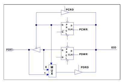
Fig. 5-27 The I/O Port and I/O Control Register Circuit
